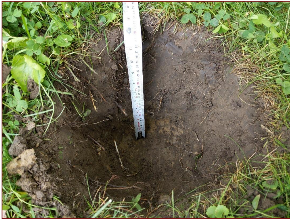
Image 6: Test Pit with Landscaping Fill over Natural Soils
