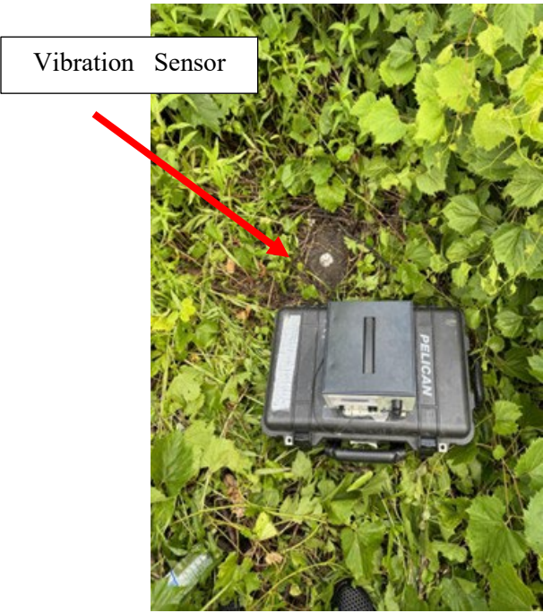
I2: Accelerometer Mounted at Measurement Location
