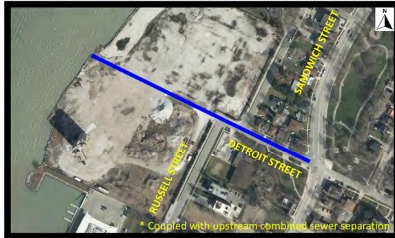
Detroit Street Trunk Storm Sewer and Outfall*
