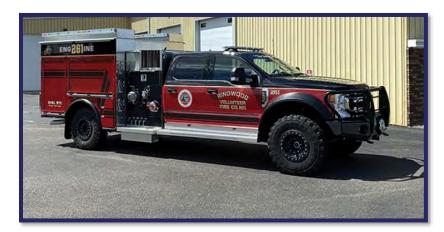
Photo: example of smaller format engine/squad with full capacity pumping capability.
