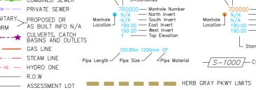
Pipe Length Pipe Size Pipe Material — S-1000 — CONSTRUCTION DWG NUMBER
