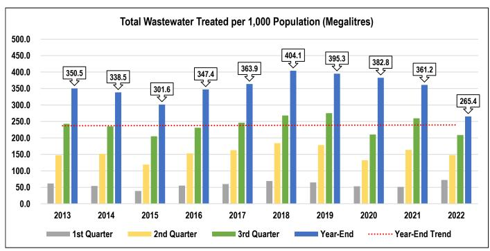
Fluctuations are partially due to changes in precipitation patterns as additional water is treated during heavy storms due to combined sewers.
