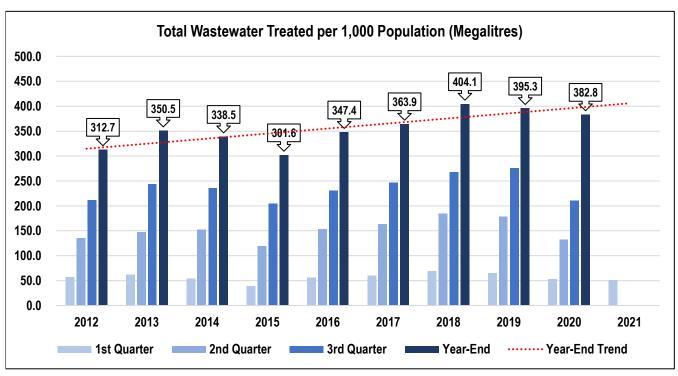
Fluctuations are partially due to changes in precipitation patterns as additional water is treated during heavy storms due to combined sewers.
