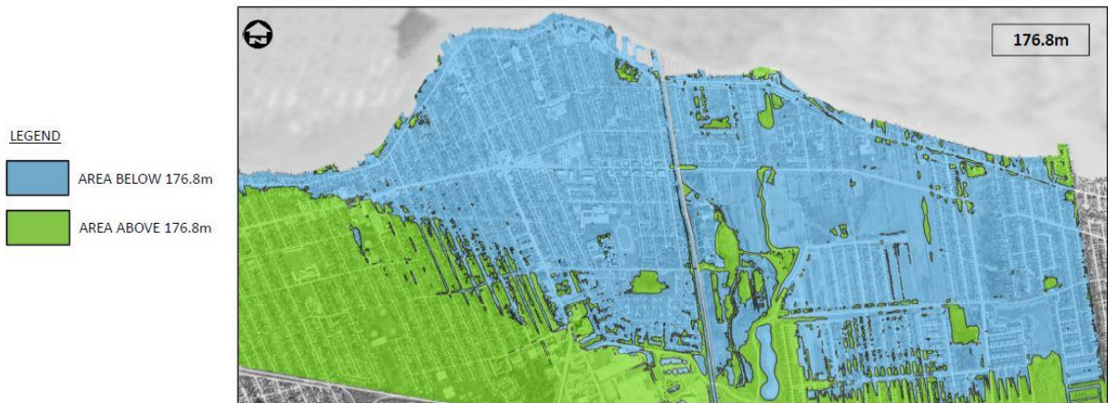
Figure 6: Area at Risk for Overland Flooding at a high water level of 176.8 m (1:100 year water level - 2050s) (Landmark Engineers, 2019)
