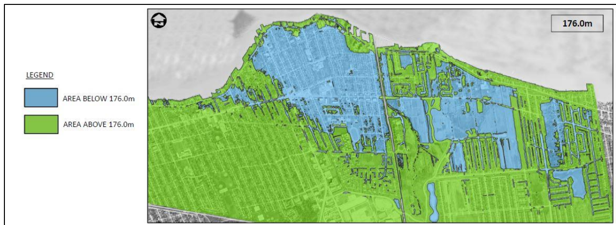
Figure 4: Area at Risk for Overland Flooding at current high water level of 176.0 m (Landmark Engineers, 2019)
